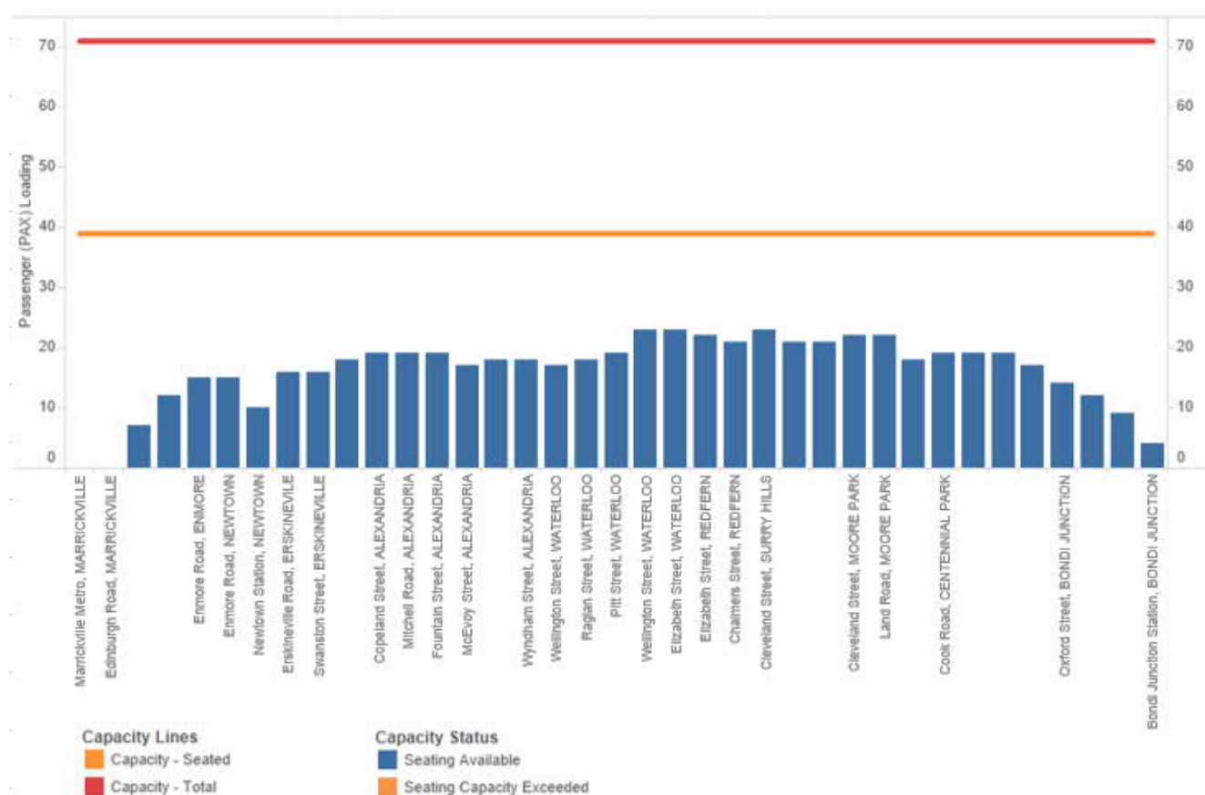
Figure 6.6: Bus service passenger loading on route 355 during the morning peak period (inbound)
